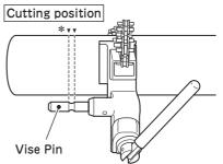
\*Cutting point varies depending on mounting position of the pipe saw.
