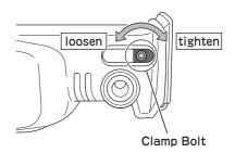
O Insert the saw blade between the Blade Holder and the Saw Guide, and put the projection of holder into the hole of blade.
