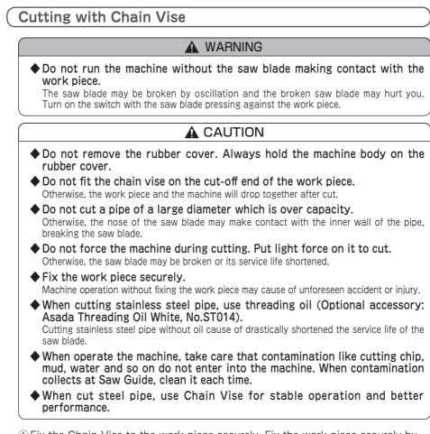
1 Fix the Chain Vise to the work piece securely. Fix the work piece securely by Vise, if the work piece is not fixed unlike installed pipe.
